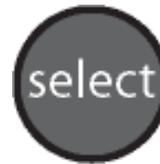
The Select Button will store all measurements in the temporary memory to the storage position shown the lower left corner of the display while in the Test Mode and while in the Menu mode it will activate an icon item or soft key.
