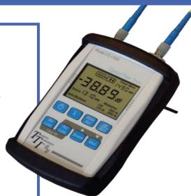
The LTS-1500 is a small, rugged automated fiber optic loss test set with a power meter that characterizes singlemode and multimode fiber links at wavelengths of 850,1300, 1310, 1490, 1550 and 1625nm and a light source with singlemode or multimode lasers. The power meter uses a sensitive InGaAs detector that is calibrated at six wavelengths with an 80+ dB dynamic range. The Light source is a single port system with up to three wavelengths.
