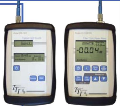
The 1500 series are small, rugged automated fiber optic Power Meters and single port Light Sources available in single, dual or triple wavelengths. The power meter uses a sensitive InGaAs detector, calibrated at six wavelengths with an 80+ dB dynamic range.
