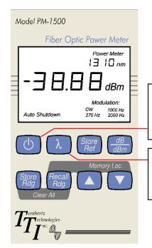
Power, ON/OFF- This control alternately energizes and de-energizes the unit. Auto-Shutdown mode, in which the unit turns itself off following fifteen minutes without a key press, is the default mode. This mode conserves the battery should the user forget to turn the unit off. Holding this key down for at least four seconds at turn-on will de-activate Auto Shutdown.
