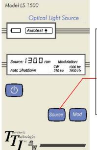
Source Selector - This control selects the laser wavelength to be used. The lasers are initially turned off when the instrument powers up. Pressing the Source button activates the laser and changes wavelength in the following sequence: 1310 nm → 1490 nm → 1550 nm, → Auto Test (in which the lasers are activated in a sequence of 5 seconds each), -> OFF.
