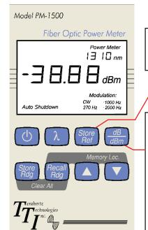
Store Reference Level- This control saves the currently measured power level for the wavelength in use. When in the dB mode, all subsequent readings will be made relative to this power level. A storage location is maintained for each of the six calibrated wavelengths.
